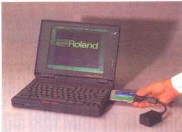
The SCP-55 plugs directly into the PCMCIA slot of a notebook computer.
